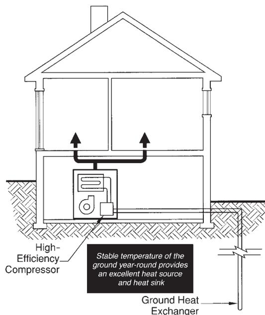
Heat pumps typically use a forced air distribution system. A fan blows air over a coil circulating the refrigerant that is either heated or cooled by the heat pump. As a result, the air is conditioned and circulated through ducts to the various spaces within a residence. A thermostat controls the system to maintain the spaces at an occupant-set temperature.
