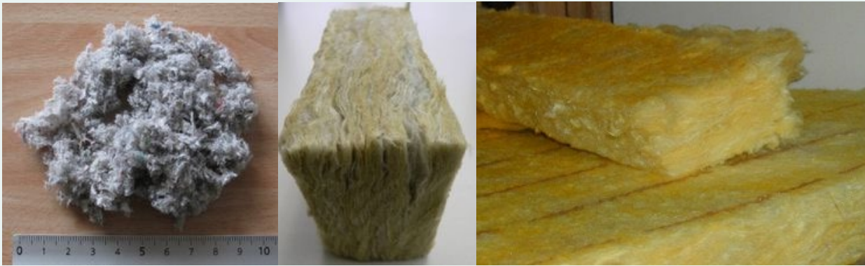
Permeable insulation examples: Cellulose, Mineral Wool, Fiberglass https://energyeducation.ca/encyclopedia/Fibrous_insulation
